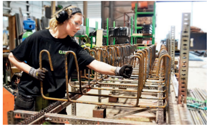
Stirrups for beams are positioned on the Skew Jig System grid
